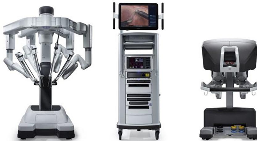
**Figure 1** The da Vinci Xi<sup>®</sup> robotic surgical system—a sample view of the robotic operating console, surgical robotic, and surgical monitor. (Intuitive, Incorporated; Sunnyvale, CA).
